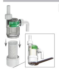
Unscrew the lower part of the neutralizer. On the lower part there is a support for a 13mm wrench to facilitate the opening
